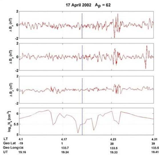
Figure 3. High-pass filtered vector magnetic field data from CHAMP in MFA coordinates and corresponding electron density data measured by PLP on April 17, 2002. The dashed line indicates the location of the dip equator.
