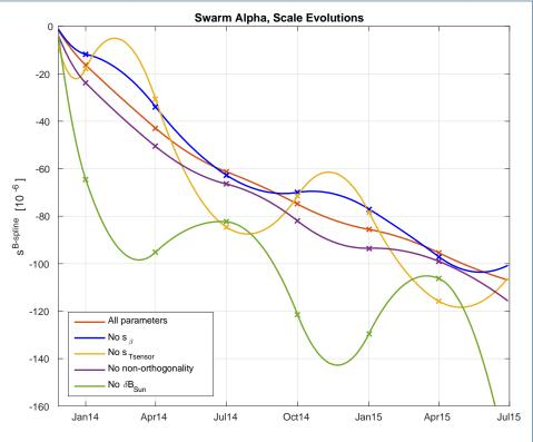
**Figure 6** Temporal evolution of estimated VFM scaling for various test models. RedGreen: full model. Blue: full model except  $s_{\beta}$ . Light brownRed: full model, except adjustment of  $s_{\mathrm{Tsensor}}$ . MagentaCyan: full model, except adjustment of VFM sensor non-orthogonalities. GreenMagenta: full model, except disturbance  $(\delta \vec{B}_{\mathrm{Sun}})$ . B-spline knots are marked with crosses.
