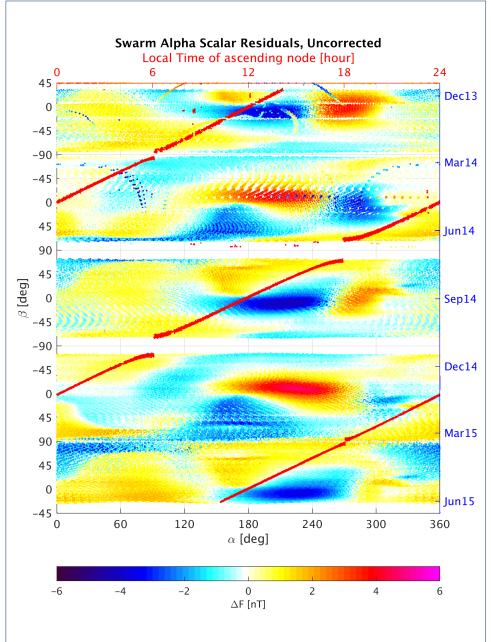
Figure 3 Uncorrected scalar residuals between ASM and VFM magnetometers,  $\Delta F$ , plotted versus Sun incident angles  $\alpha$  and  $\beta$ . The  $\beta$  angle oscillates slowly in time, hence the *un-folded*  $\beta$  angle corresponds to season which is indicated in blue on the right hand side. Local Time of the ascending node is shown in red (axis on top).
