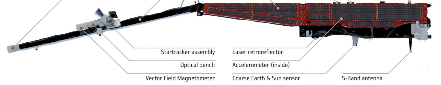
The two science magnetometers on Swarm are the Absolute Scalar Magnetometer (ASM) at the tip of the boom and the Vector Field Magnetometer (VFM) 1/3 inwards on the boom. Around both magnetometers are the white, thermal blankets made of an outer layer of betacloth and multiple aluminum layers beneath. Also noticeable is the thermal blanket on the bottom side of the boom, a.k.a. the "boom-blanket".
