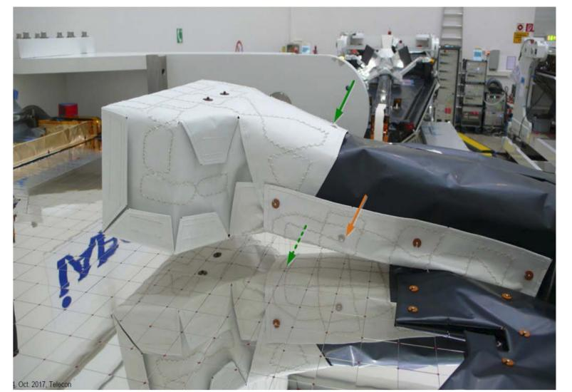
which are electrically connected both through the grounding network as well as through the thermal blankets, hence currents will flow in the blankets and grounding wires in close proximity to the magnetometers. The differences in the estimated  $dB_Sun$ 's (cf plots at the bottoom of this poster) of the three spacecraft can be explained by differences in resistances, mainly contact resistances and resistances in the aluminum foils of the thermal blankets.
