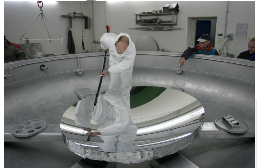
FM Primary Reflector coated with aluminum. Shown in aluminizing plant.
