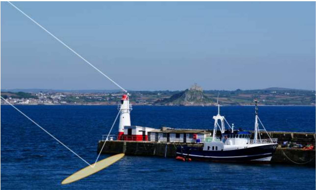
Figure 1. The direct and reflected GNSS signal for a GNSS receiver on a pier.
