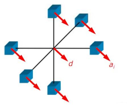
Gradiometer = 6 Accelerometers, each accelerometer measures
