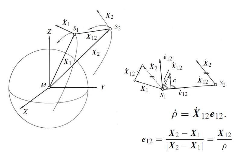
Fundamental observation is velocity range rate ty Or velocity change **along**  $e_{12}$  **called**  $\vec{\rho}$
