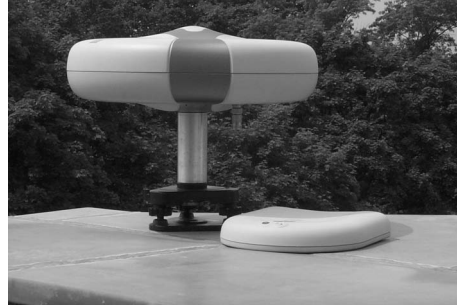
Figure 7.97. Combined GPS-GLONASS receiver JPS Legacy with RegAnt antenna
