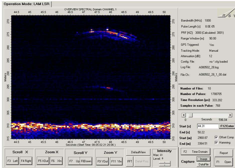
Figure 15. “Quicklook” image of helicopter over-flight on May 2<sup>nd</sup>. Note the reflection from both the helicopter itself and the EM bird below it
