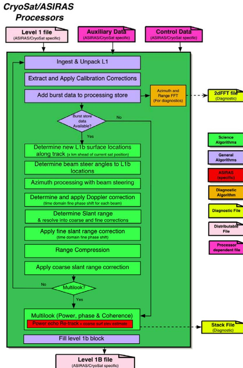
Figure 10. ASIRAS processing scheme.
