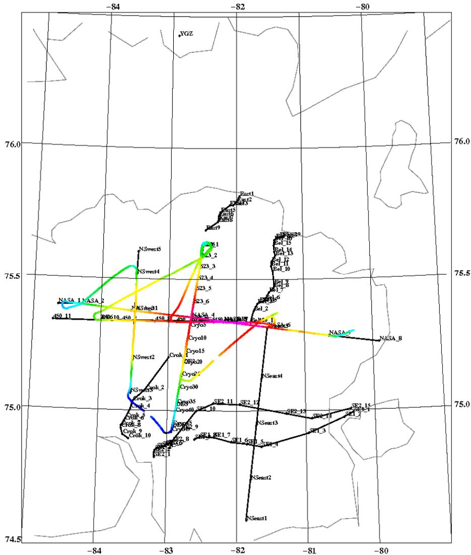
Figure 16. Laser scanner swaths of the Devon Ice Cap survey on May 6<sup>th</sup> (colour coded heights relative to the WGS84 ell.). (In black: The planned lines – some on opportunity basis and not all observed)
