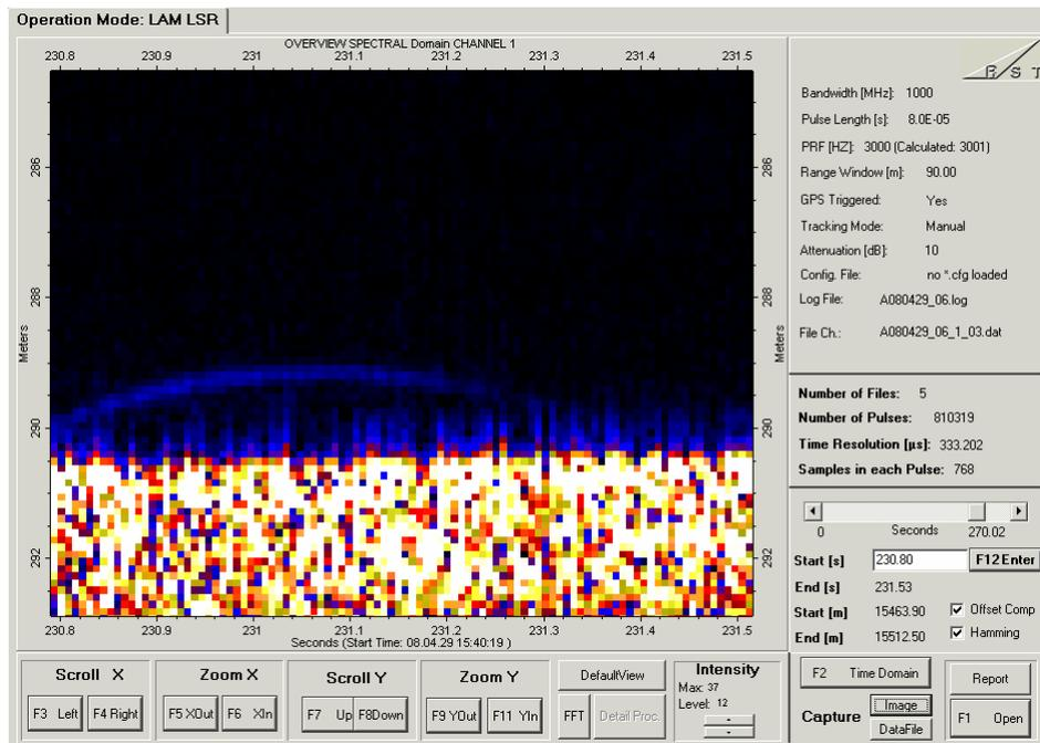
Figure 12. “Quicklook” image showing radar signal from the corner reflector at ICE2
