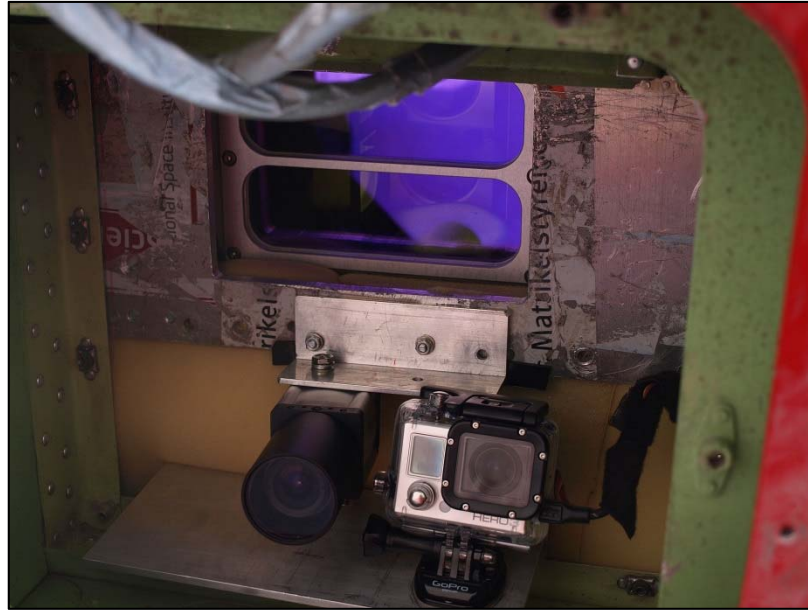
Figure 9: Camera installation of nadir-looking cameras for CryoVEx 2016; uEye (left) and GoPro (right).
