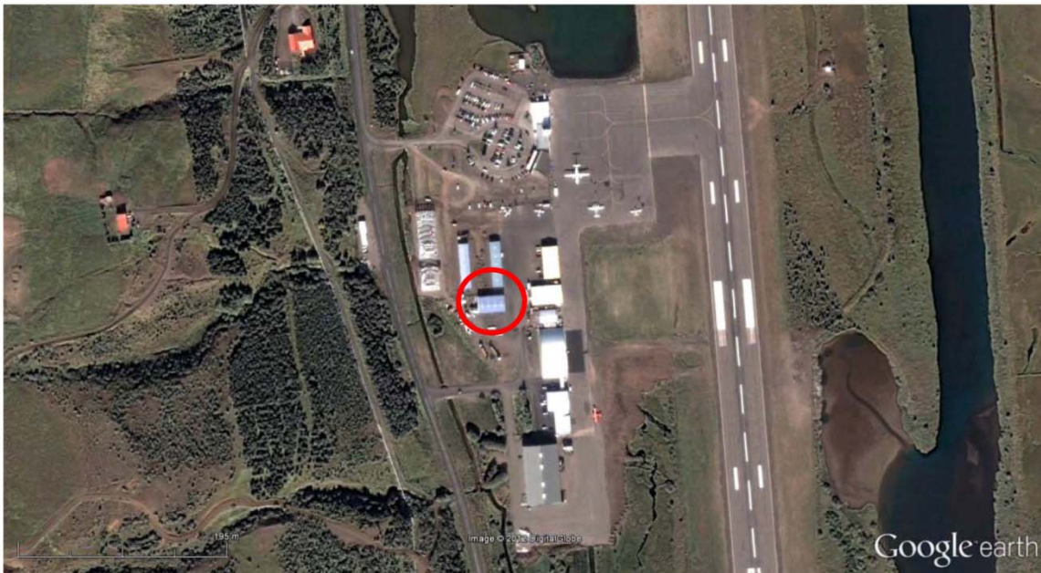
Figure 8: Map of Akureyri airport with building used for calibration marked by red circle. The corners of a building close to the Norlandair hangar and the runway were surveyed by geodetic GPS to be included in the calibration of the ALS and ASIRAS. The scanner image is shown in appendix D.
