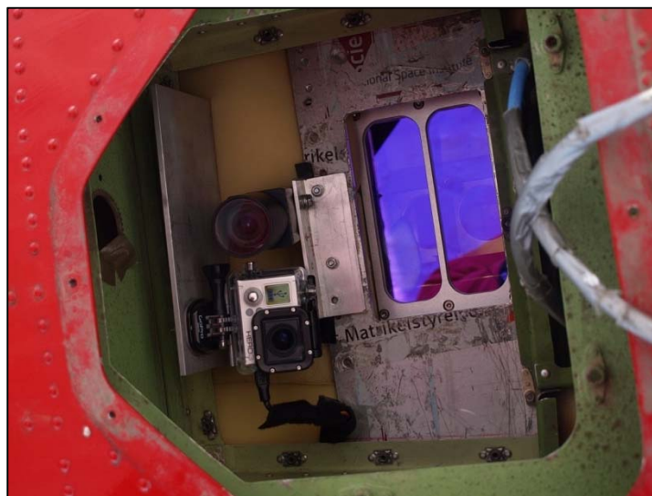
Figure 6 Instrument bay in rear baggage compartment of the aircraft. In front laser scanner RIEGL LMS Q-240i with heater pads (grey/orange instrument). H-764G INS (grey box) and OXTS INS (red box) in the back. Between the two INS instruments are mounted two external heaters.
