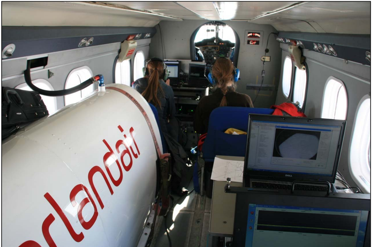
Figure 4 View of cabin in aircraft; Rack with ASIRAS PC's (front right), rack for ALS, GPS and INS (rear left). Spare fuel tank for extra airborne time (front left) Photo: SSIM.
