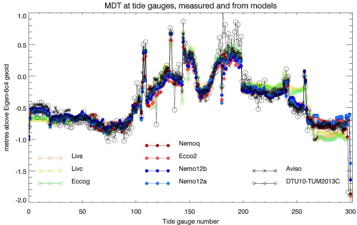
**Figure 7: The MDT at 302 tide gauges (black circles) using the Eigen-6C4 geoid to its full resolution, compared with predictions from 7 ocean models (colours), and 2 satellite-derived MDTs (black).**
