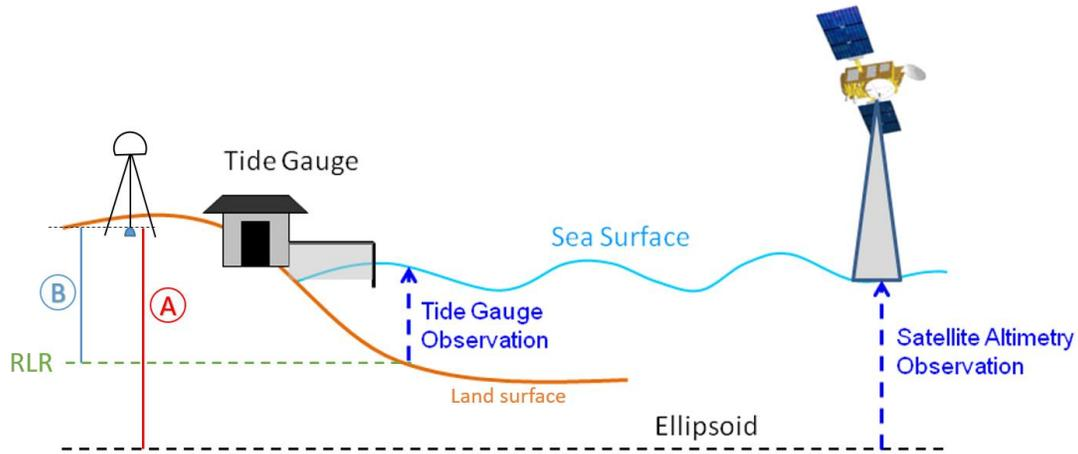
Figure 1: Basic references and quantities at a TG-GNSS collocation site
