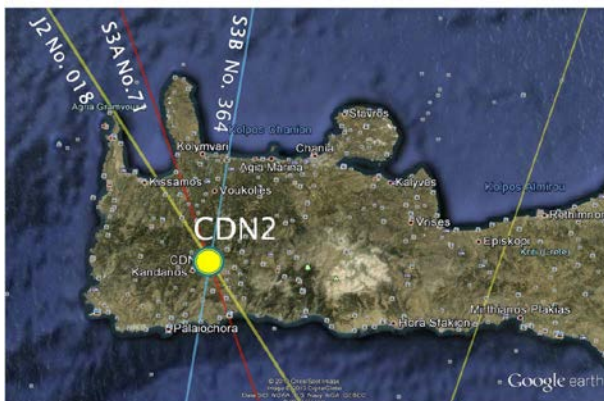
Figure 7. A triple cross-over point for Sentinel-3A (red), -3B (purple) and Jason series (yellow) exist at the CDN2 site in western Crete.
