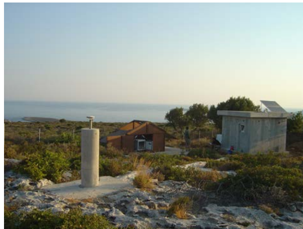
Figure 8. The GNSS receiver next to the transponder at the SLR2 site in west Crete. A similar infrastructure is to be constructed at the CDN2 site.
