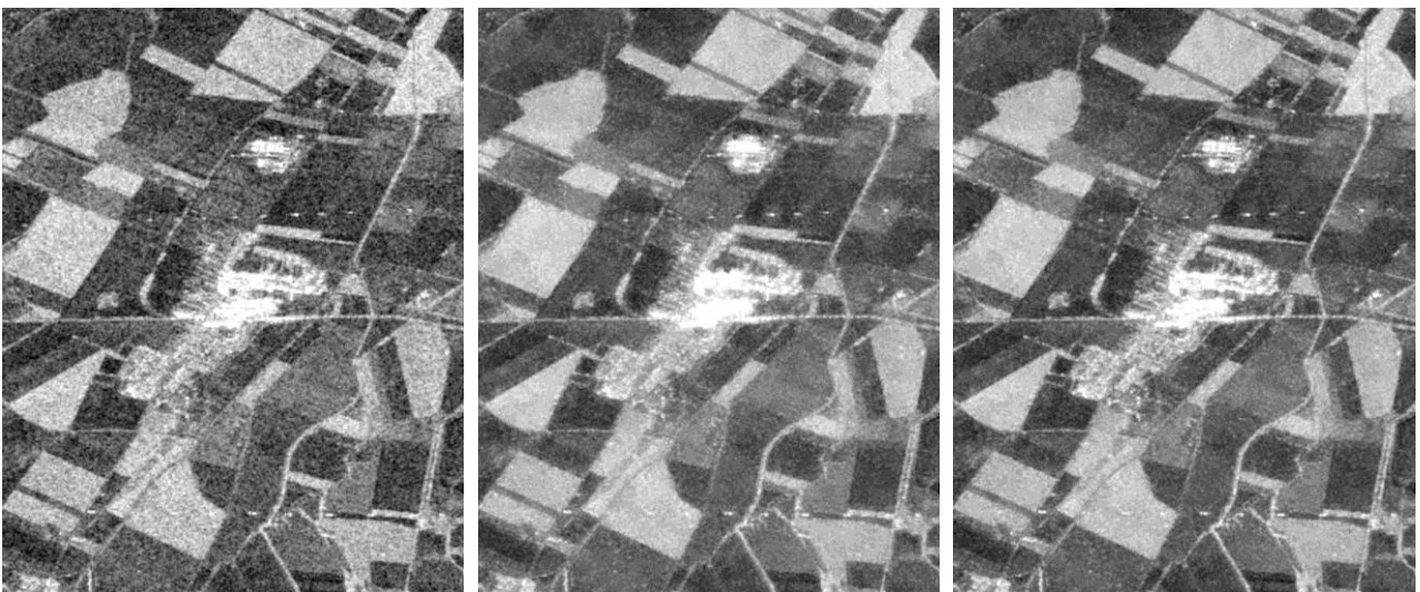
Figure 5 Unfiltered (left), spatially filtered (center) and filtered using the presented advanced multi-temporal filter(right) PALSAR data for a 4km x 6km section in Hungary.
