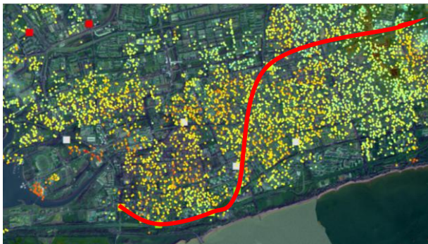
Figure 3. Vertical land deformation in Marine Parade area (red rectangle on Figure 2). Levelling marks (coloured squares) and profile in red.
