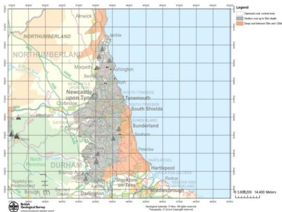
Figure 1. The Northumberland and Durham coalfield; depth of coal shown by colour; Grey <50m, orange >50m.
