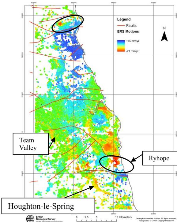
Figure 3: ERS (1995 to 2000) derived motion for the Northumberland region. Black circles on the image highlight motion phenomenon which appear to be bounded by the major faults in the region shown in red. Sites mentioned later are highlighted by text.
