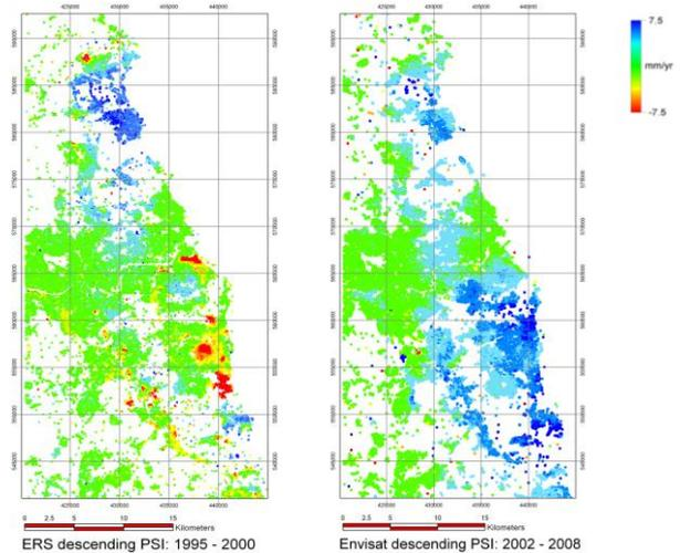
Figure 2. InSAR results, average annual velocities, for the Northumberland region, left shows deformation from 1995 to 2000 and right shows deformation from 2002 to 2008. Blue indicates surface uplift and red colours indicate surface subsidence. (InSAR data © NPA Satellite Mapping, a CGG Company; SAR data © ESA).
