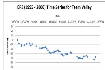
Figure 4: ERS 1995-2000 PSI data for the team valley and Terrain motion time series for the cluster highlighted by black circle
