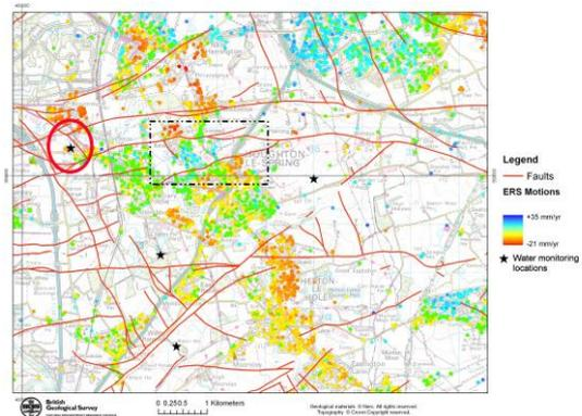
a. ERS motion in the Houghton area, red lines are faults and red circle highlights the area for which the Figure 3b graph is drawn. Black dashed rectangle highlights area shown in more detail in Figure 3c.
