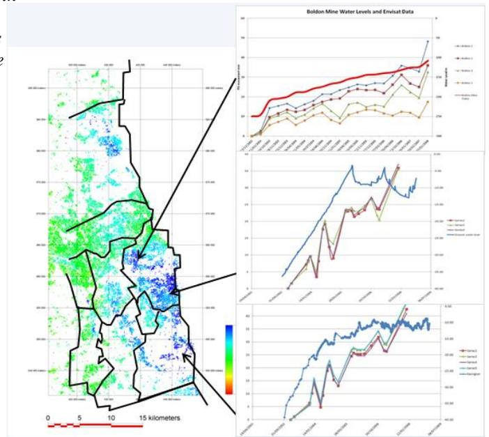
Figure 7: Minewater recovery curves (thick blue and red lines) compared with PSI derived ground motions for the monitoring stations highlighted by arrows.
