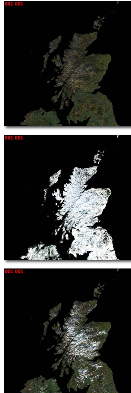
Figure 4. State estimates over Scotland, shown as BHR RGB true colour composites for snow-free (top), snow (middle), and actual (bottom) conditions. DOY 1 2005.
