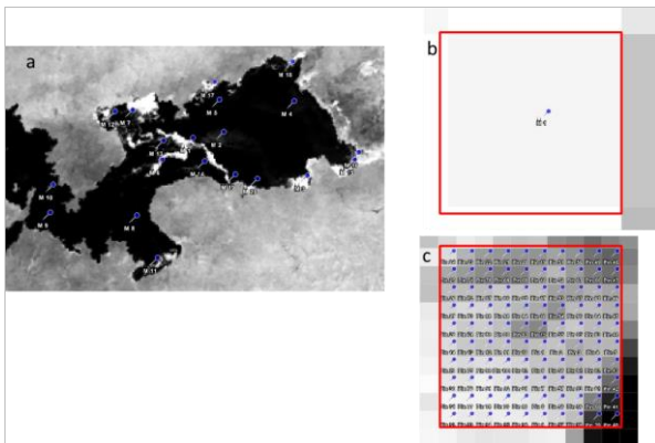
Figure 4. (a) Location of the 20 randomly selected sample pixels, (b) M1 MERIS pixel (300 m), (c) Corresponding 100 Landsat TM pixels (30 m)
