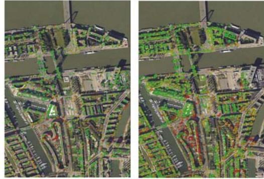
Figure 1. Envisat versus TerraSAR-X point density. On average, a tenfold increase in point density is obtained by switching from medium (Envisat) to high resolution (TerraSAR-X) satellite data.
