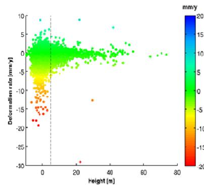
Figure 2. Ground/building separation based on estimated heights of persistent scatterers (Envisat, 2003-2010). A threshold of 3 m above ground level was chosen to distinguish between high and low points.
