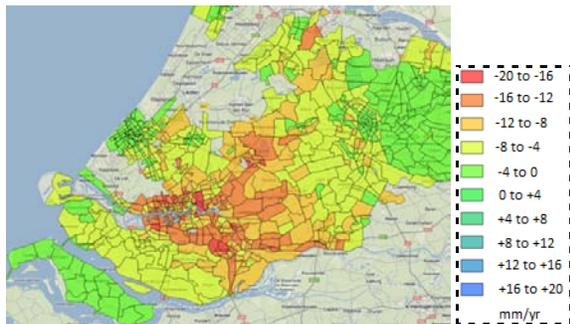
Figure 4. Wide area differential subsidence rates (Envisat, 2003-2010). Polygon boundaries correspond to the Dutch postal codes. Colors denote the representative value for the linear deformation rate. The 10<sup>th</sup> percentile is used in this case. Only ground points are included in the analysis.
