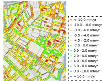
Figure 5. Deformation analysis along pipeline routes. Colors denote estimates of averaged linear deformation rates (in mm/yr). Results are presented for points 10 m spaced along the pipelines. Weighted averaging of points within 25 m of the pipes is performed.
