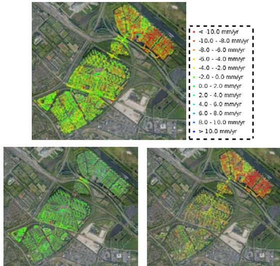
Figure 3. Linear deformation rates (TerraSAR-X, 2009-2012). Upper panel: all PS; Lower left: PS on buildings with a deep foundation, resulting in stability. Lower right: ground level. The difference with the left image shows the differential motion of the top soil layer adding stress to pipelines.
