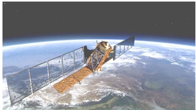
Figure 1. Artist's View of Sentinel-1 with Deployed Solar Arrays and SAR Antenna
