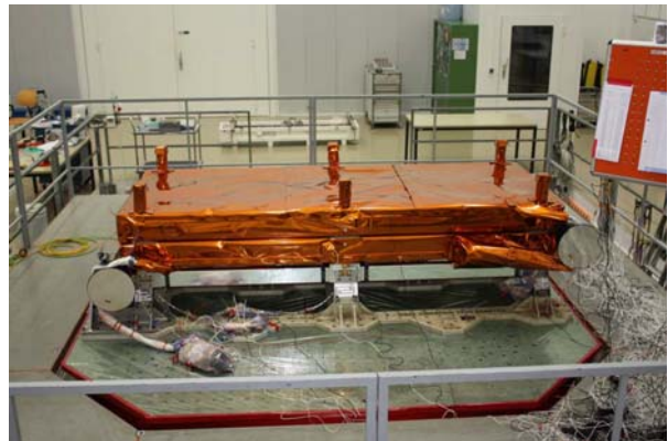
Figure 13. Vibration Test: SAS -X Wing Mounted on Shaker
