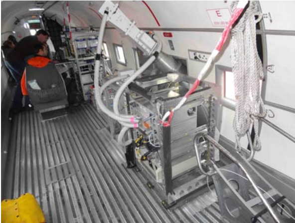
Figure 3. EMIRAD and antennas inside the aircraft
