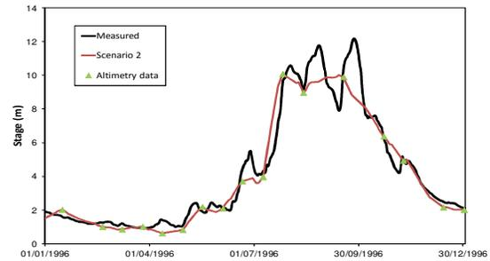
Figure 4. Measured and estimated stage data at Nakhon Phanom for 1996. The measured data was only used for validation
