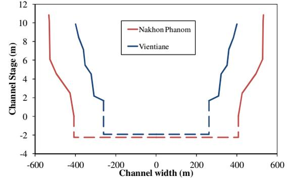
Figure 6. Channel cross-sections (solid lines) and bathymetric depths (dashed lines) for a 50km reach on the Mekong River.
