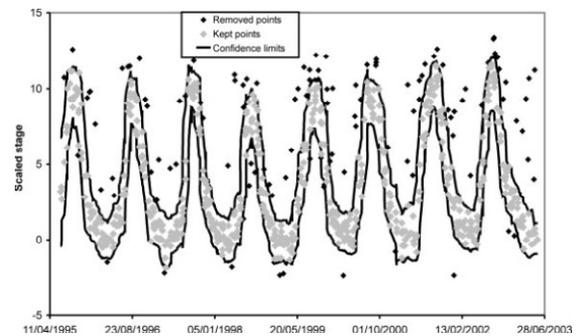
Figure 2. Rejected points, accepted points and confidence bounds for the ERS-2 altimetry data
