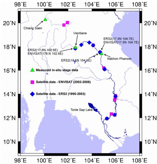
Figure 1. Measured in situ stage and satellite altimetry data on the Mekong River.
