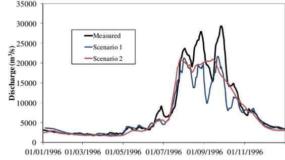
Figure 3. Measured and estimated discharge at Nakhon Phanom for 1996. The measured data was only used for validation
