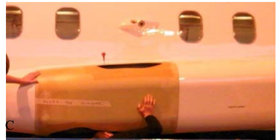
Figure 4: A) Aircraft blister on the side of the FAAM BAe146-301 aircraft which can house 3 instruments. B) ISMAR installed into the front bay. C) The front bay with the ISMAR fairing cover installed prior to painting.
