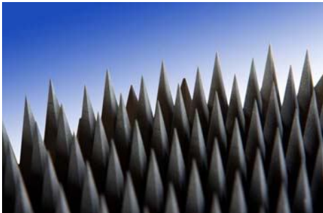
Figure 7: Pyramidal structure of the black body targets in ISMAR, designed and manufactured by RAL.
