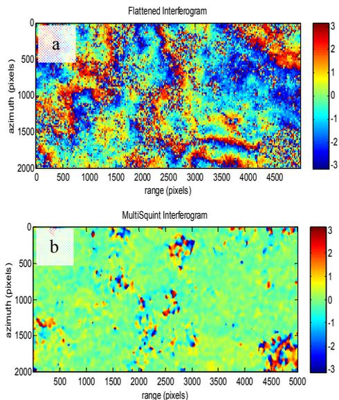
Figure 7. MS analysis on TSX data affected by a strong APS.
