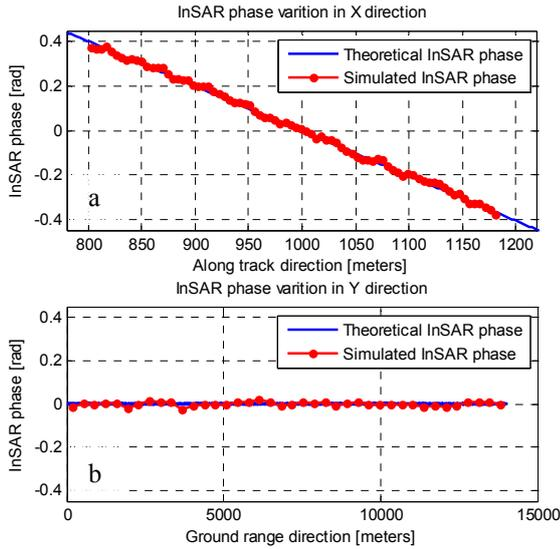
Figure 2. InSAR phase in along track direction (linear orbit error).
