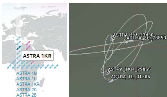
Figure 4. Left: SES constellation of COMSATs at 19.2^\circ E , right: examples of ground tracks of orbits.
