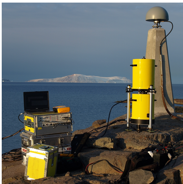
Figure 1: The A10-019 at the Thule GNET GNSS antenna (THU3) in 2009.
