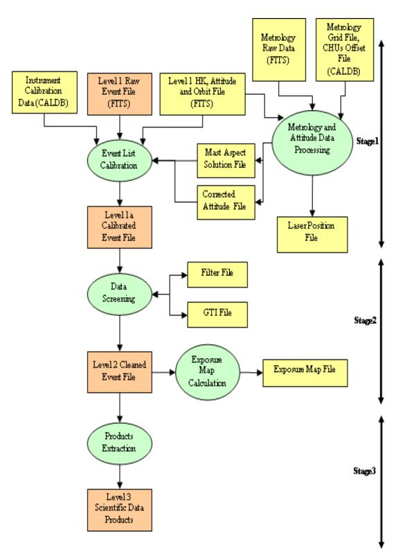
Figure 1: NuSTARDAS data reduction flow diagram
