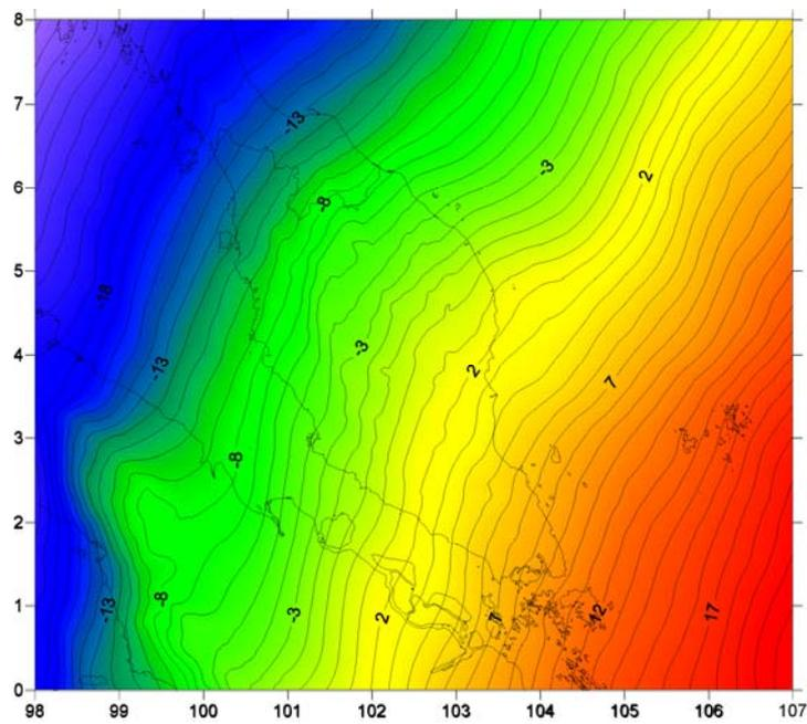
Fig. 4b. Final gravimetric geoid for peninsular Malaysia (WMG03C). Contour interval 1 m.
