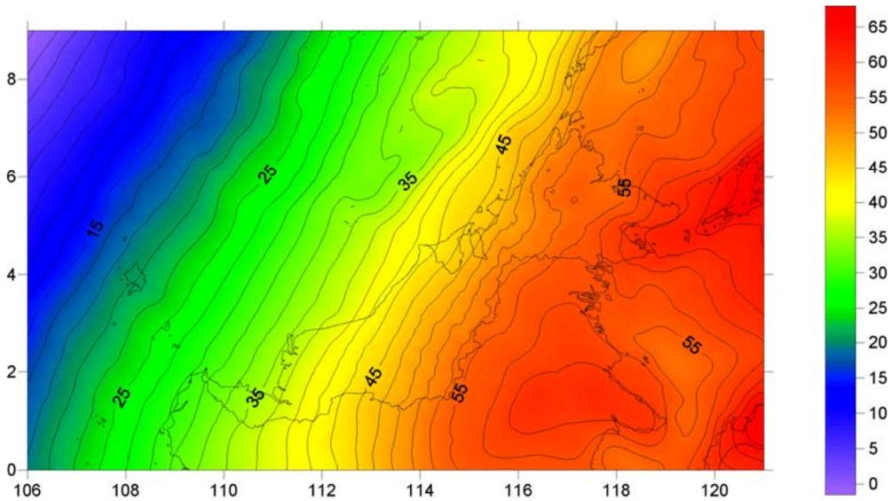
Fig. 4a. Final gravimetric geoid for East Malaysia (EMG03A). Contour interval 2 m.
