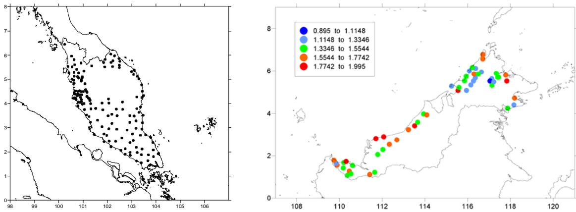
Fig 5. GPS/levelling data in West (left) and East Malaysia (east, with offset  $N^{GPS} - N$  in colours).
