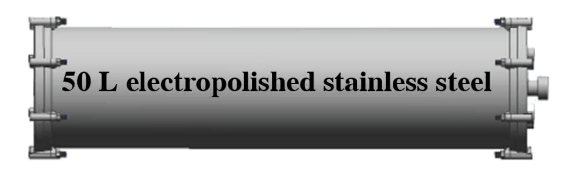
We used a 50 L electropolished stainless steel chamber. Collimated UV light entered through a Teflon foil to start the oxidation of SO<sub>2</sub> into sulfuric acid that condense with water to form aerosols. Aerosols and trace concentrations of ozone and SO<sub>2</sub> were measured along with temperature, pressure, and humidity. A continuous flow of 3.1 L/min of clean, humidified, synthetic air went through the chamber, which was kept at 1 mbar overpressure at all times.
