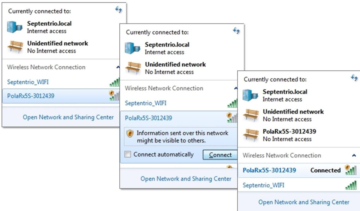
**Figure 3-7:** Select the PolarX5S from the list of detected wireless signals and connect
