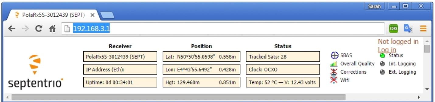
**Figure 3-5:** Connect to the Web Interface of the PolaRx5S over USB using the IP address **192.168.3.1** on any web browser
