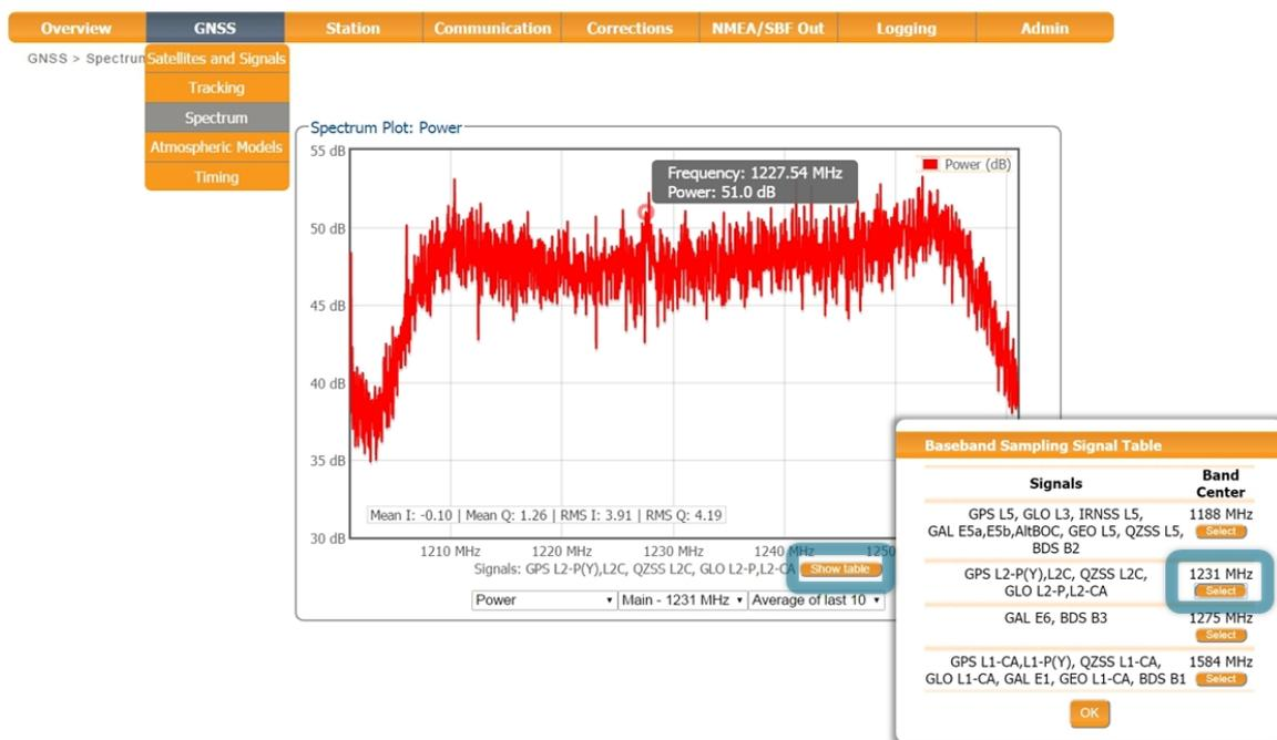
Figure 5-2: The RF spectrum of the L2 Band
