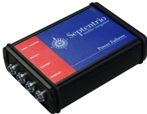
The optional power failover is a power source switch which automatically switches over to a 12 V battery backup supply during outages of the main power supply. The typical setup is depicted in Figure E-2.
