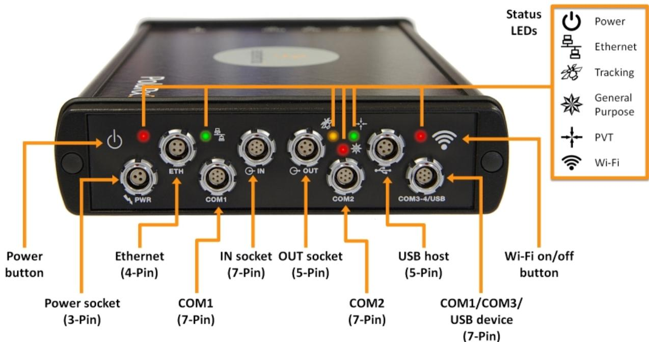
Figure 2-1: PolARx5S front-panel layout
