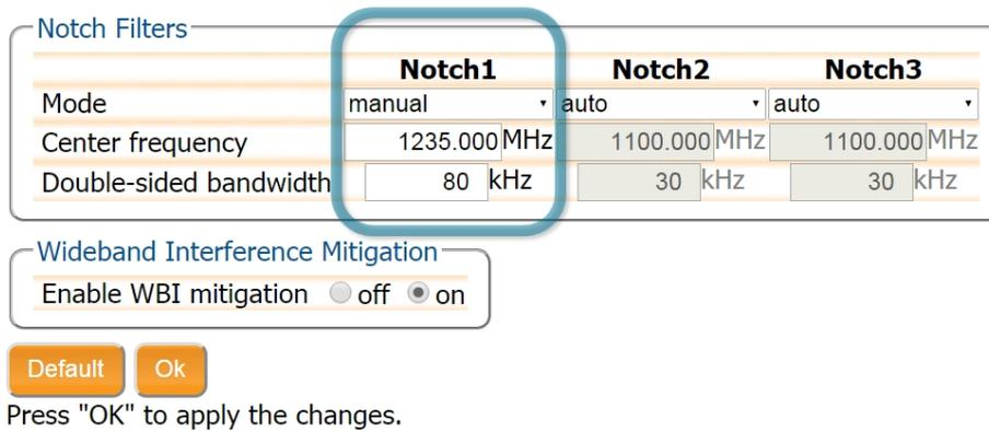
**Figure 5-3:** Configuring the first notch filter Notch1 at 1235 MHz
