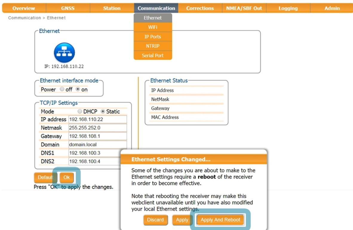
The screenshot shows the web interface for configuring the PolaRx5S. The 'Communication' menu is selected, and the 'Ethernet' sub-menu is active. The current IP address is 192.168.110.22. The 'Ethernet interface mode' is set to 'Power on'. The 'TCP/IP Settings' section is configured for 'Static' mode with the following values:
