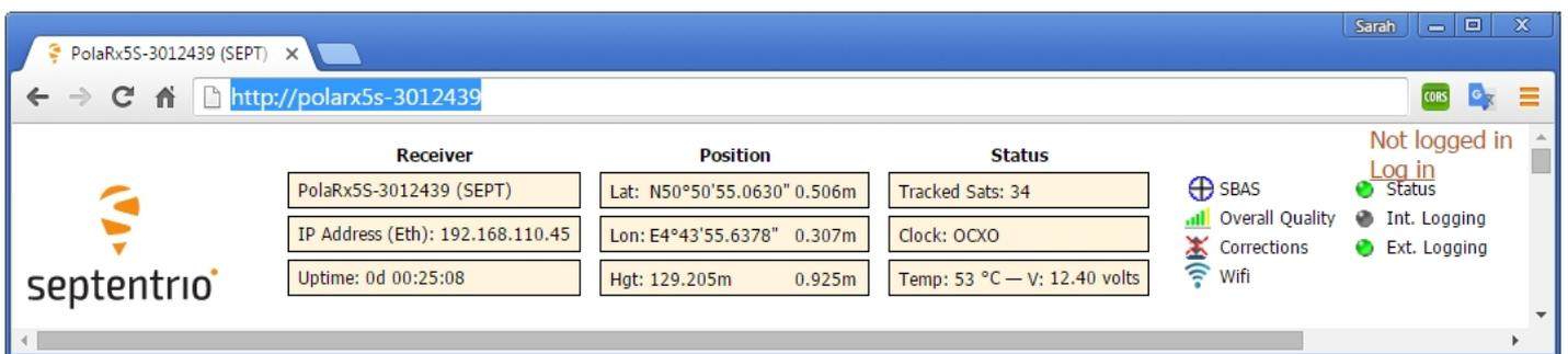
**Figure 3-10:** Connecting to the Web Interface over Ethernet
