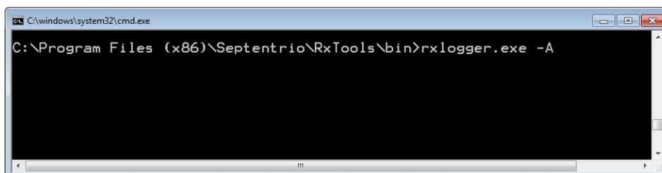
**Figure 4-14:** Launching RxLogger from the command line
