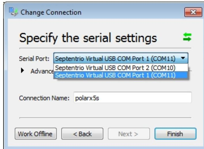
**Figure 4-1:** Connecting to the PolRx5S over USB using RxLogger
