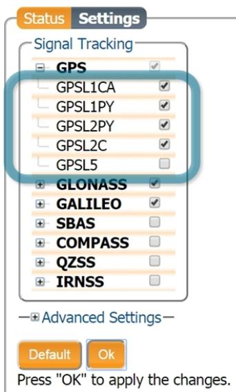
**Figure 7-2:** Configuring the receiver not to track the GPS L5 signal
