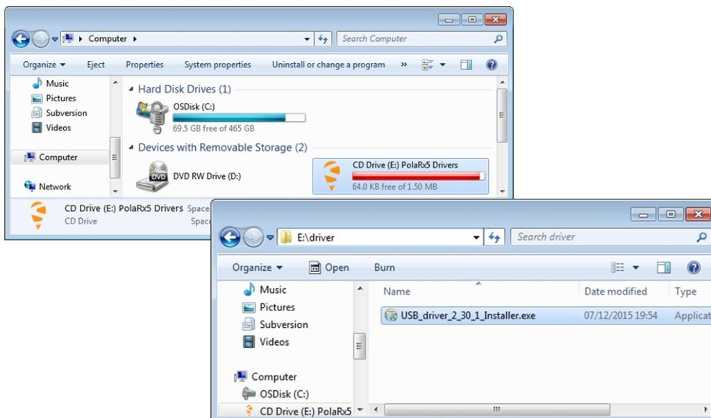
**Figure 3-4:** Manually installing the USB drivers
