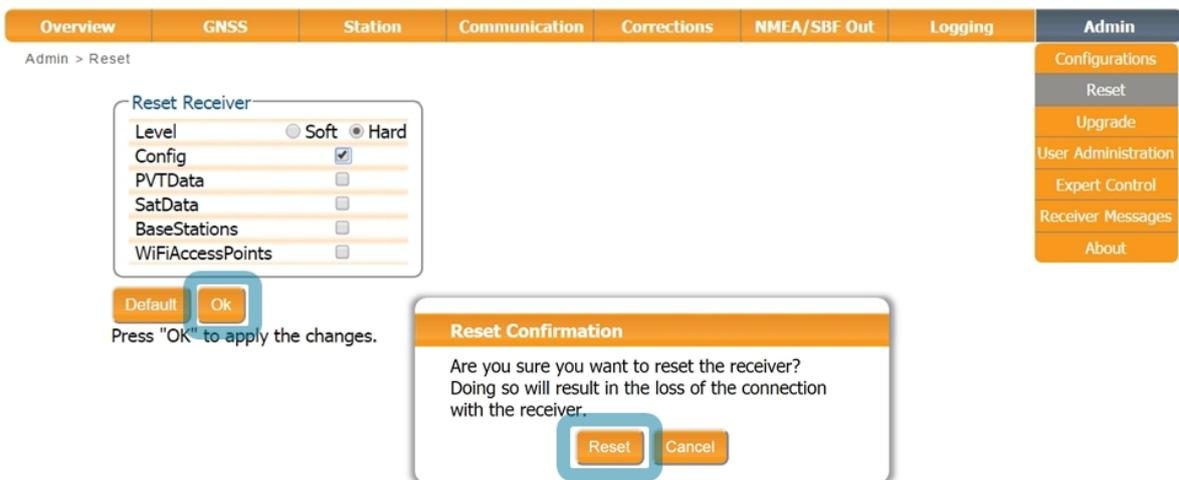
Figure 7-10: Resetting the PolaRx5S configuration to its boot configuration using a Hard reset
