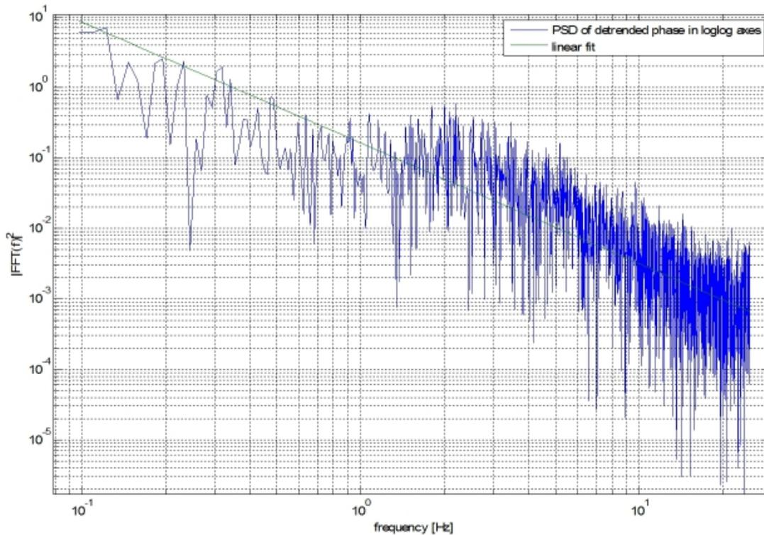
Next to the spectral slope, the spectral strength (often noted ' $T$ ') is provided in columns 60 to 62. The spectral strength is the detrended phase power spectral density at 1.0 Hz, i.e. the intercept of the linear polynomial described above.
