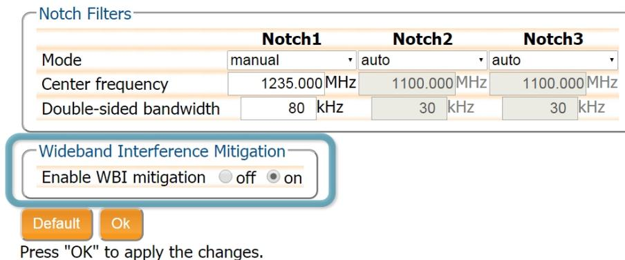
**Figure 5-5:** Select 'on' to enable wideband interference mitigation then 'OK' to apply the new setting
