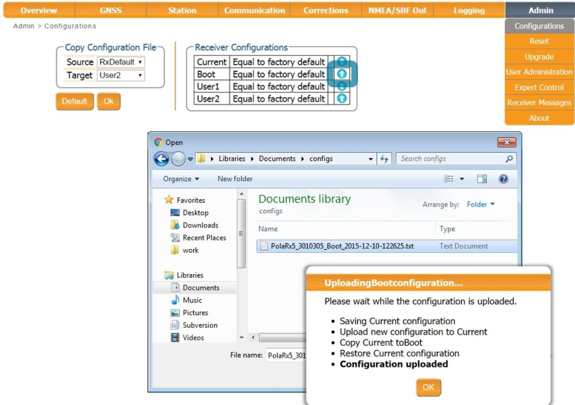
Figure 7-12: Uploading a configuration to a PolaRx5S
