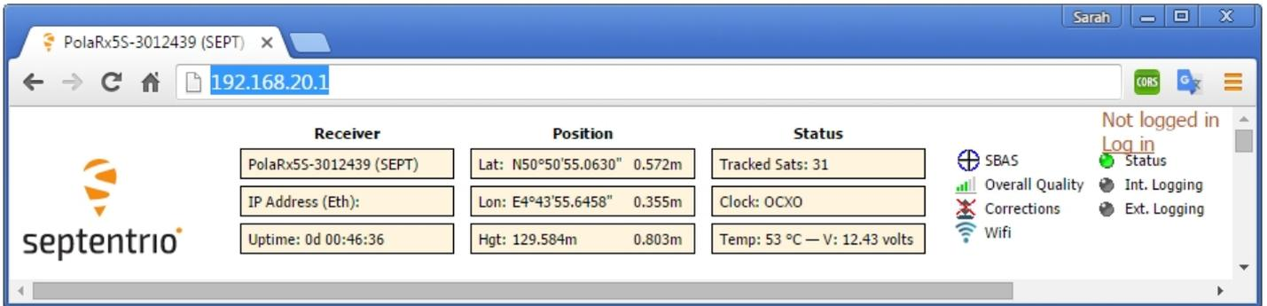
**Figure 3-8:** Connect to the Web Interface of the PolARx5S over WiFi using the IP address **192.168.20.1** on any web browser
