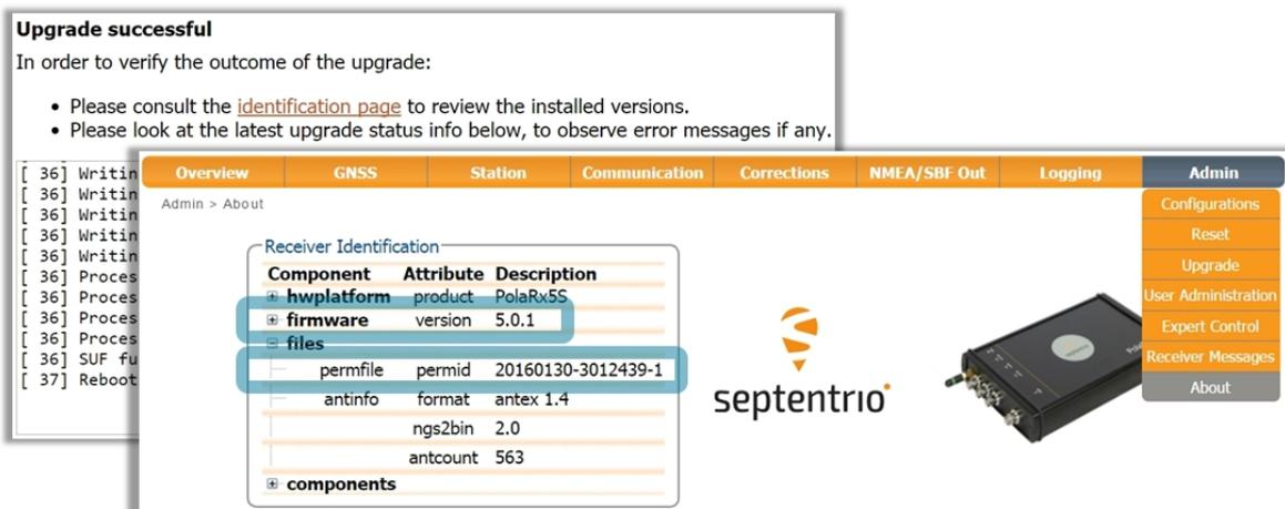
Figure 7-8: Checking the firmware and permission file versions
