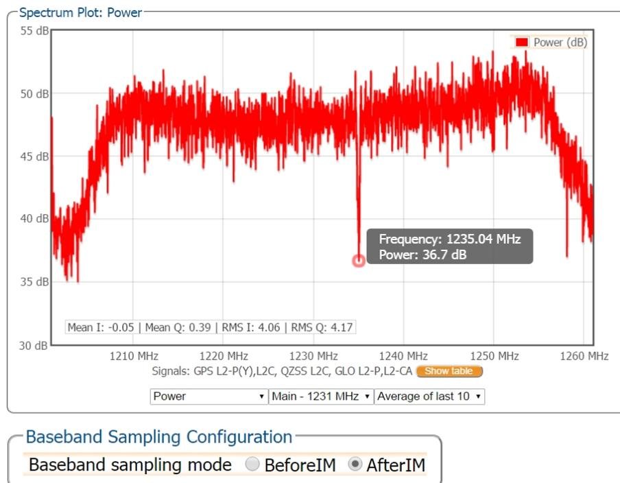
**Figure 5-4:** The RF spectrum of the L2 Band after applying the notch filter at 1235 MHz
