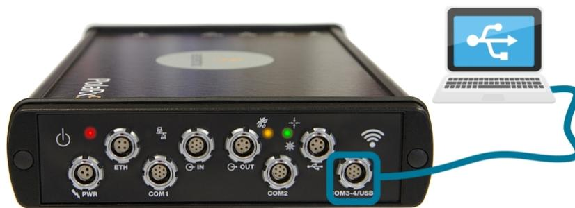
**Figure 3-3:** Connecting to the front-panel USB socket
