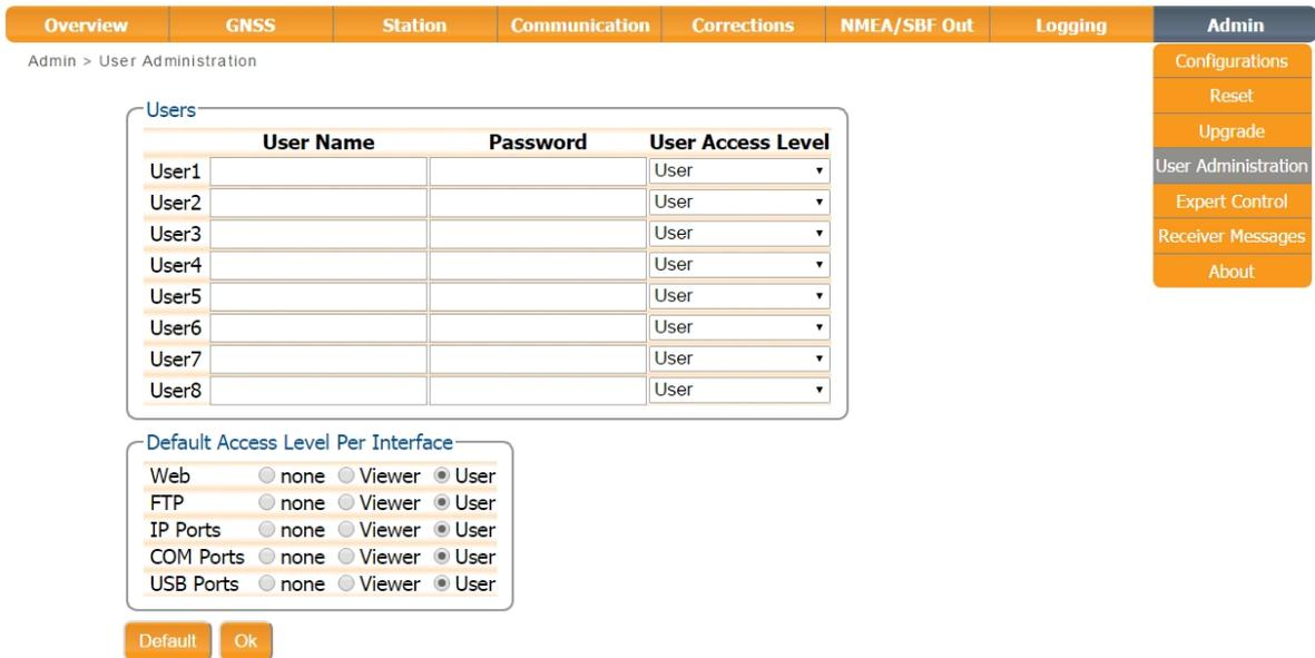
The screenshot shows the 'Admin' menu with 'User Administration' selected. The 'Users' table lists eight users, all with 'User' access levels. Below the table is a 'Default Access Level Per Interface' section with radio buttons for 'none', 'Viewer', and 'User' for Web, FTP, IP Ports, COM Ports, and USB Ports. All are set to 'User'.
