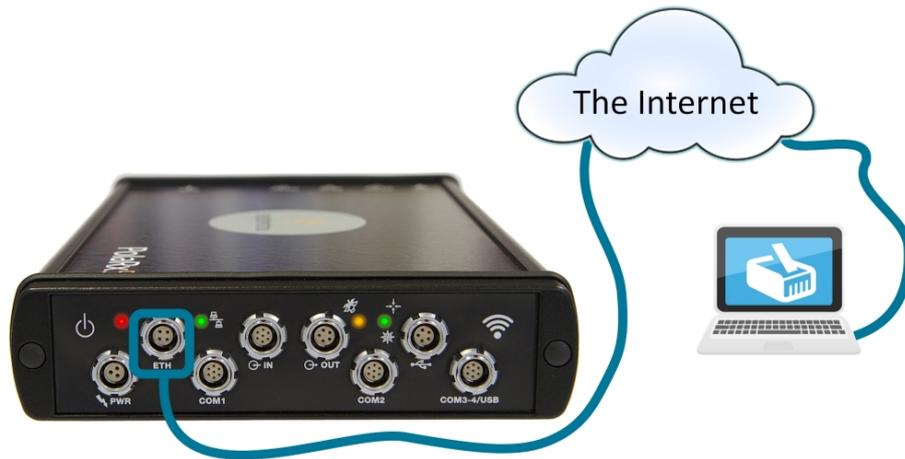
**Figure 3-9:** Connecting to the front-panel Ethernet socket
