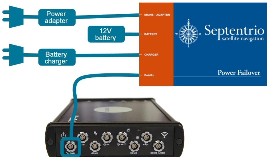
**Figure E-2:** Typical setup of the power failover with the PolARx55
