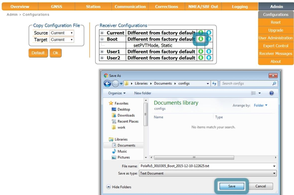
Figure 7-11: Saving a configuration from a PolaRx5S as a text file
