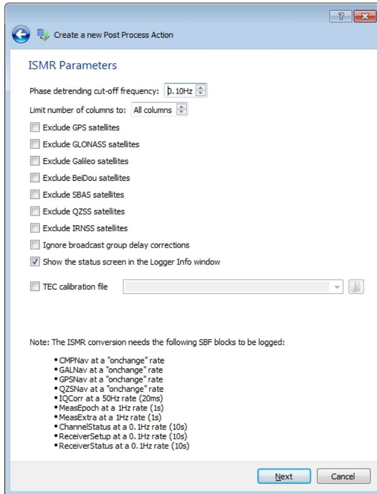
**Figure 4-7:** The default parameters for SBF conversion to ISMR
