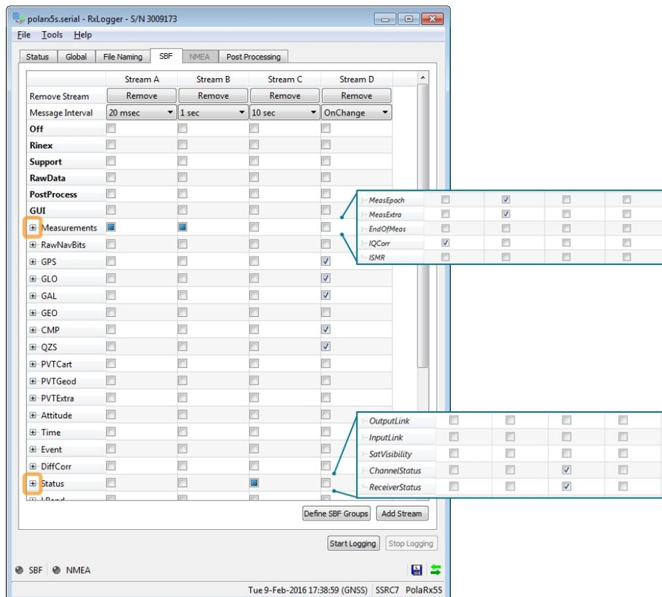
**Figure 4-5:** Select the SBF blocks and logging rates needed for ISMR file generation
