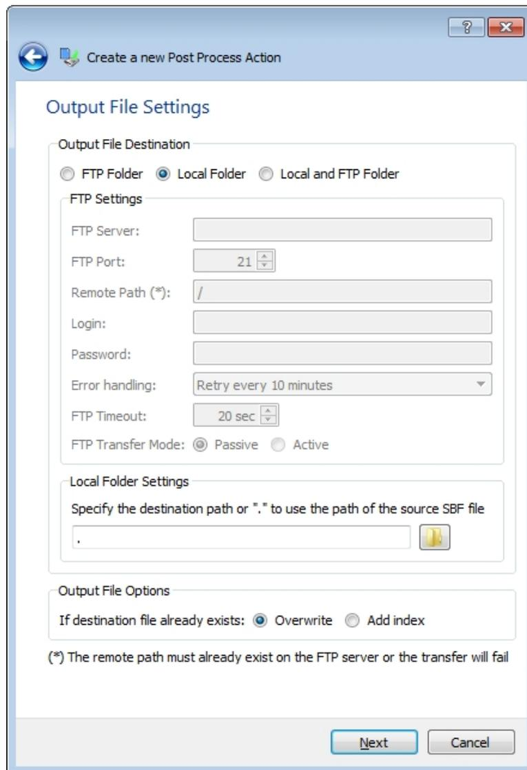
**Figure 4-9:** Storing the generated ISMR files in the default location - alongside the logged raw SBF files
