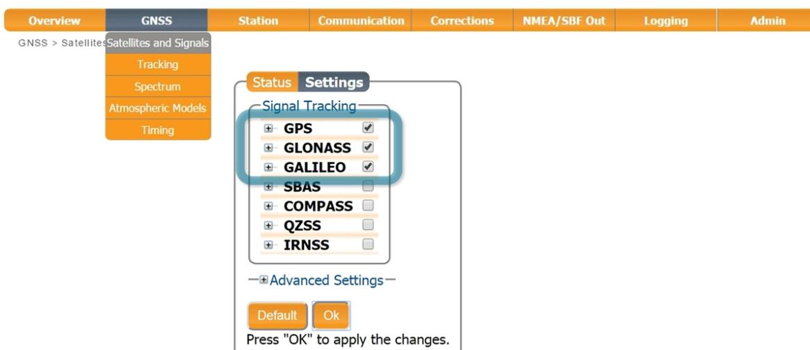
**Figure 7-1:** Configuring the receiver to track only satellites from the GPS, GLONASS or Galileo constellations
