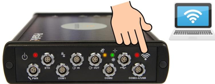
**Figure 3-6:** Press firmly on the front-panel WiFi button
