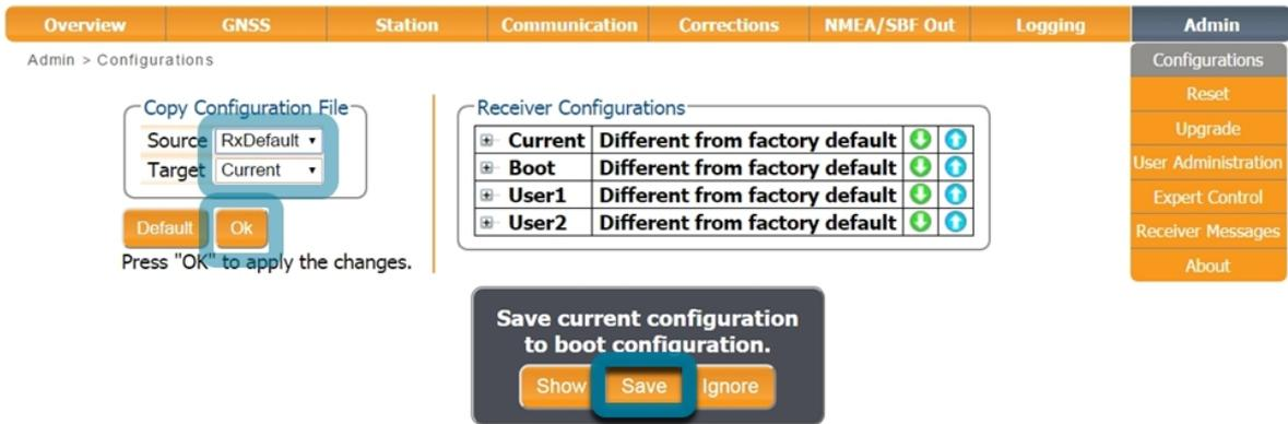
Figure 7-9: Setting the PolaRx5S to its default configuration
