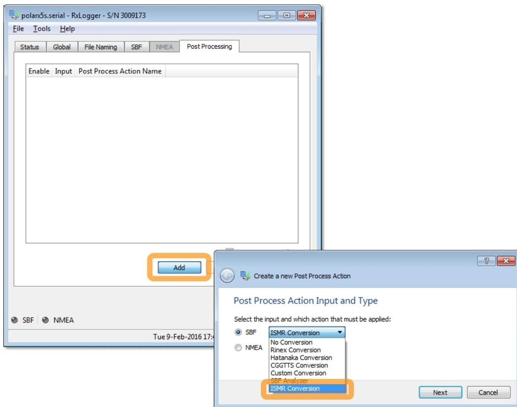
**Figure 4-6:** Selecting automatic generation of ISMR from SBF data files
