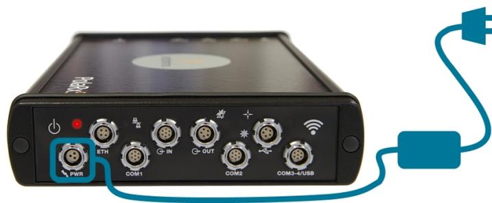
Figure 3-1: Front-panel power socket
