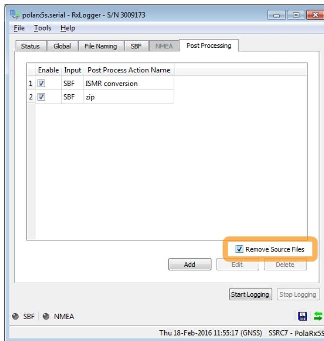
**Figure 4-13:** Select 'Remove Source Files' to delete the non-compressed raw SBF files after generating the compressed files
