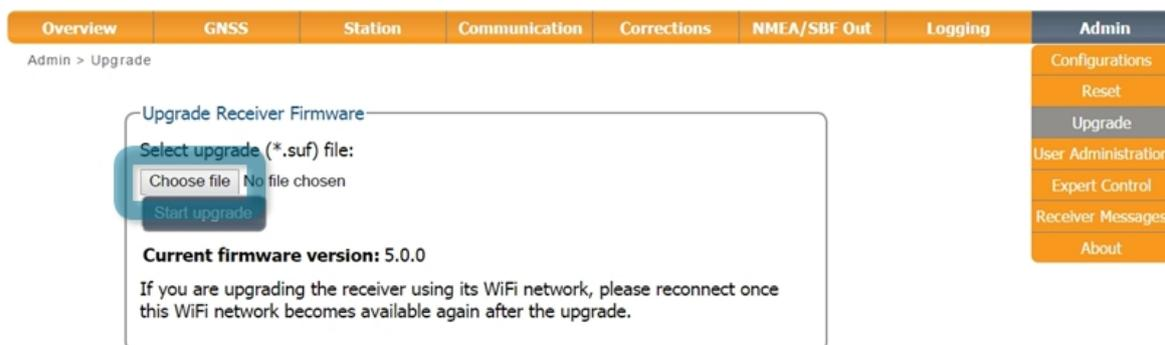
**Figure 7-6:** Selecting the .suf file to upload to the receiver
