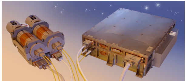
Fig. 11 ^4\text{He} magnetometer from LETI (by courtesy of J.-M. Leger)
