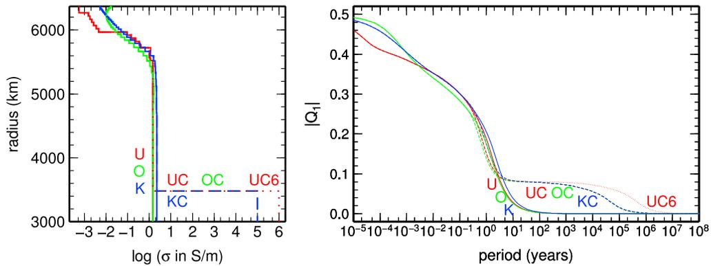
**Figure 1.** (left) Spherically symmetric conductivity models U, O, and K (red, green, and blue solid lines, respectively), models including a conductive core, UC, OC, and KC (red, green, and blue dashed lines, respectively), and model UC6 using upper estimate of core conductivity (red dotted line). (right) Corresponding amplitudes of  $\tilde{Q}_1$  responses as functions of period.
