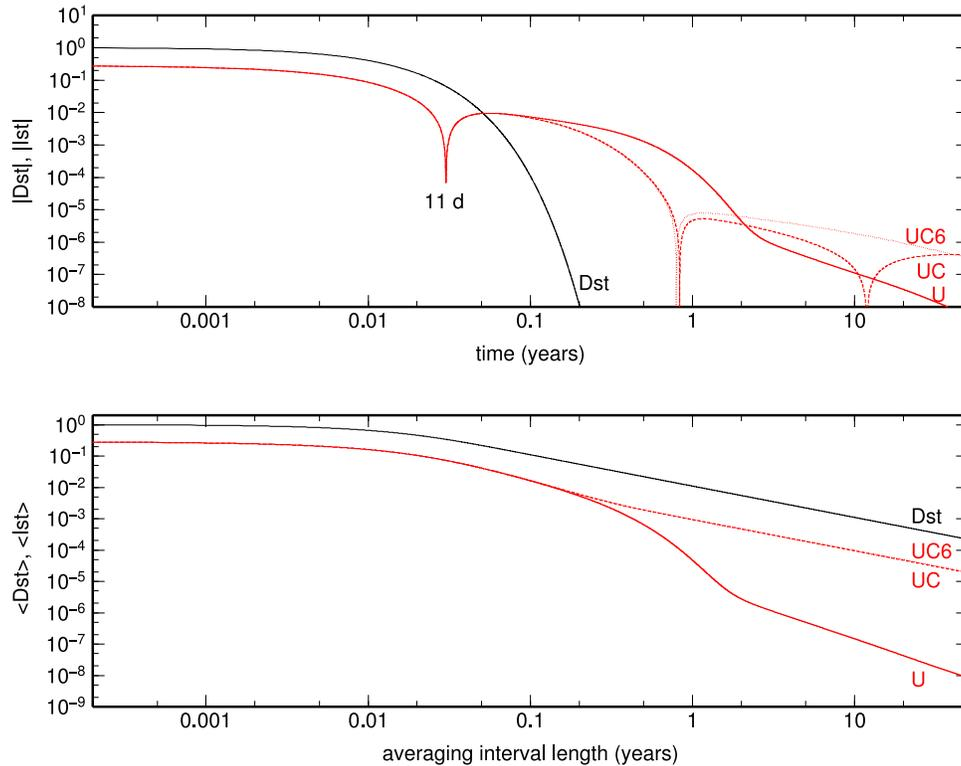
**Figure 2.** Induction by the exponential synthetic storm model. (top) The  $D_{st}(t)$  index and the  $I_{st}(t)$  indices obtained for conductivity models U, UC, and UC6, respectively. (bottom) The dependence of average values of  $D_{st}(t)$  and  $I_{st}(t)$  on the length of averaging interval. Synthetic  $D_{st}(t)$  is shown in black, and synthetic  $I_{st}(t)$  is in red, using solid, dashed, and dotted lines for respective conductivity models.
