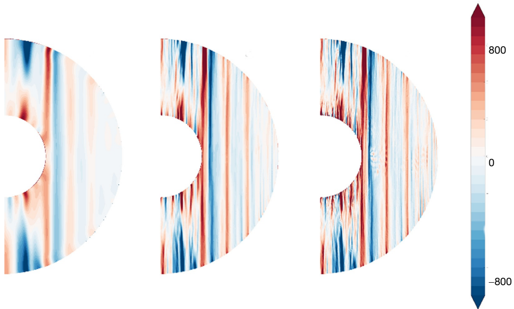
Figure 2 Quasi-geostrophy of velocities with large scales in directions at right angles to the rotation axis. A meridional slice (snapshot) of the azimuthal velocity extracted from a rapidly rotating dynamo model driven by mass anomaly flux at the two boundaries (see, e.g., Aubert et al., 2009) with p_m=0.1 and Ekman number \nu/\Omega(r_c-r_i)^2=10^{-7} , leading to Rossby number Ro\sim 6\times 10^{-4} and Lehnert number \lambda\sim 10^{-3} . Less and less small scales are filtered out from left to right, illustrating the progressive loss of quasi-geostrophy as the length scale is decreased. Left and middle: scales respectively smaller than 0.1r_c and 0.02r_c are filtered out. Right: full solution. Personal communication from N. Schaeffer (see also Chapter 8.06).
