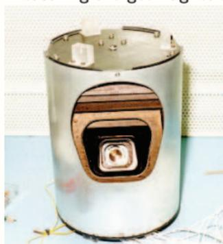
**Fig 2.12:** Examples of a satellite fluxgate magnetometer (left) and star cameras (right) for measuring instrument orientation.
