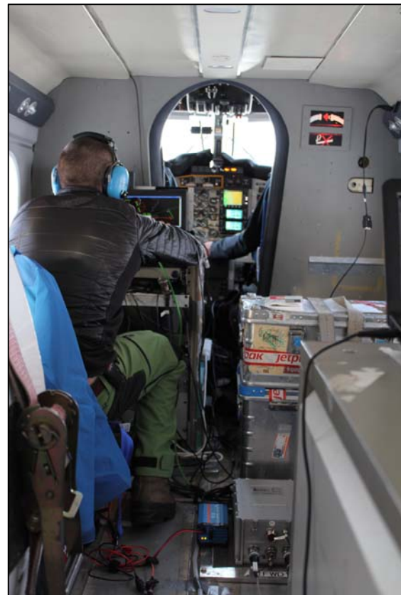
Figure 5: View of cabin in aircraft; Left picture: Rack with Ka-band altimeter (front right), rack for ALS, GPS and INS (rear left). Right picture: iMAR strap-down INS, grey box attached to the floor (lower right).
