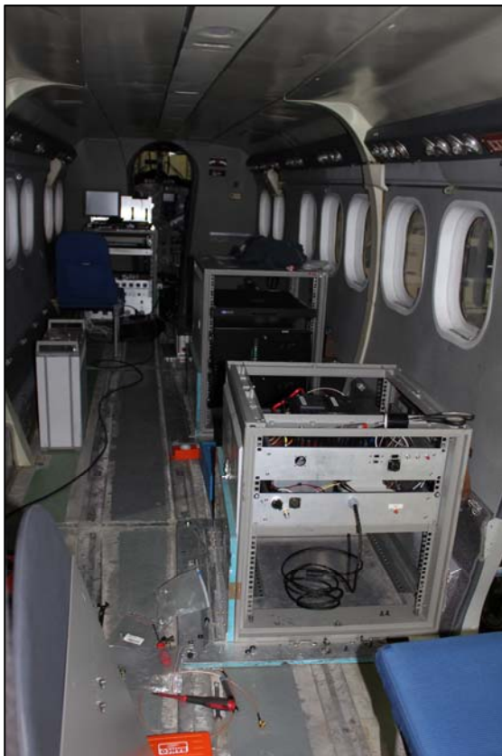
Figure 5: View of cabin in aircraft; Left picture: Rack with Ka-band altimeter (front right), rack for ALS, GPS and INS (rear left). Right picture: iMAR strap-down INS, grey box attached to the floor (lower right).
