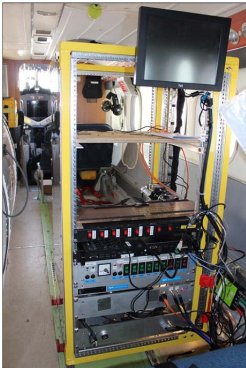
Figure 11: Rack setup in BAS Twin Otter VP-FAZ. All instruments are fitted in one rack see image on the left from below; KAREN altimeter, power unit, rack PC to support Honeywell INS, and another power unit. Control PC's are shown in right image from below; ALS (left), camera (right), KAREN, Honeywell INS.
