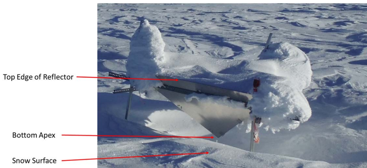
Figure 24: Photo of corner reflector at Devon ice cap covered in snow by courtesy: D. Burgess, Natural Resources Canada
