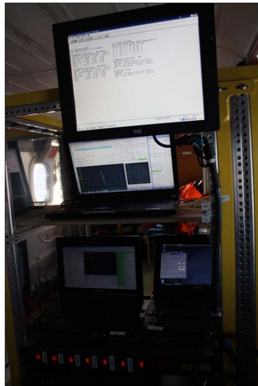
Figure 11: Rack setup in BAS Twin Otter VP-FAZ. All instruments are fitted in one rack see image on the left from below; KAREN altimeter, power unit, rack PC to support Honeywell INS, and another power unit. Control PC's are shown in right image from below; ALS (left), camera (right), KAREN, Honeywell INS.
