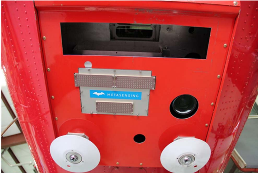
Figure 10: Bottom view of the BAS Twin-Otter VP-FAZ showing KAREN, ALS together with radiometers and camera.
