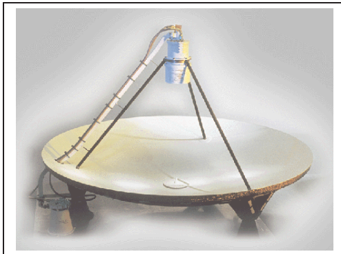
Figure A.2: The ENVISAT radar altimeter is a parabolic antenna (Source: See chapter 8).
