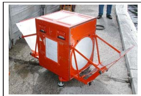
Figure F.2: Transponder ready for operation. The sides can be upfolded to ease transportation. The weight is about 85 kg.
