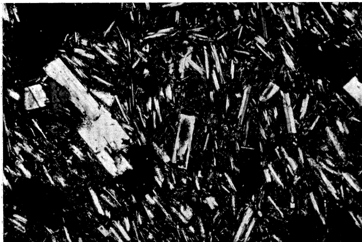
FIGURE 74. Trachyandesite (183). Flow from Hill-with-a-hole-in. Phenocrysts of zoned plagioclase An_{60} to An_{37} in sub-parallel orientation and microphenocrysts of pyroxene in a groundmass of plagioclase, pyroxene, alkali feldspar, ore and glass. Crossed polars. (Magn. \times 34 .)
