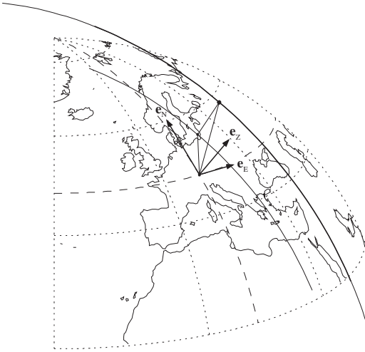
Fig. 2.12. Satellite motion in the local tangent coordinate system. Only the part of the orbit which is marked by a bold line, and the corresponding ground track, are visible from the given station
