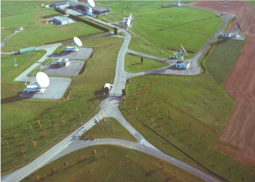
Fig. 1.8. The ground station complex at Redu, Belgium, provides telemetry, tracking, and telecommand operations for low-Earth and geostationary satellites (courtesy ESA)
