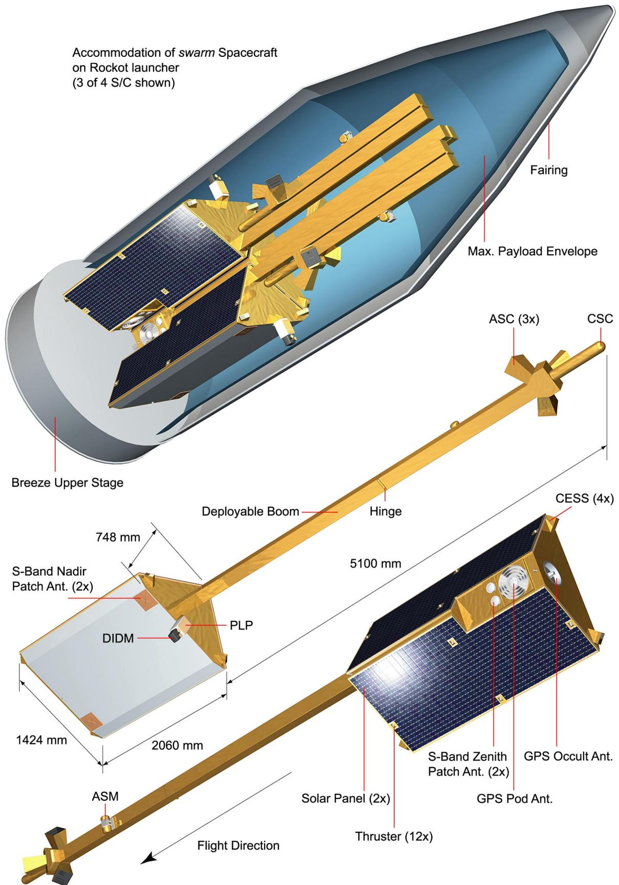
Figure 3.4: *swarm* satellite configuration and accommodation in Rockot fairing
