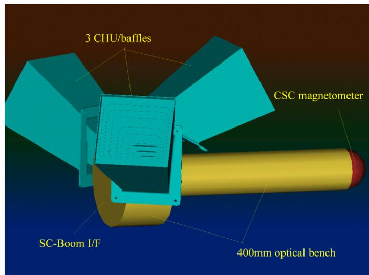
Figure 3.2: Optical bench mounted with triple CHU and CSC
