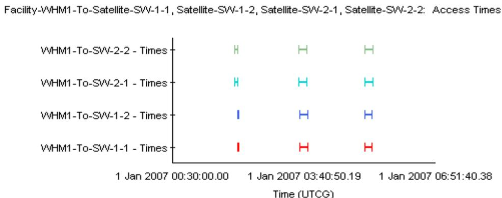
*Figure 3.11: Typical ground station coverage patterns for swarm during LEOP*
