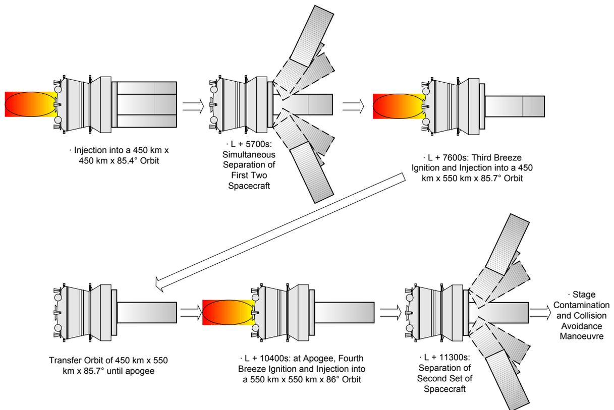
Figure 3.9. Rockot Flight Sequence for injecting swarm satellites into the required orbits
