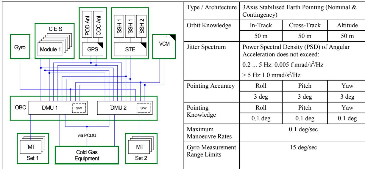
Figure 3.7: swarm AOCS Architecture and Main Performance Data
