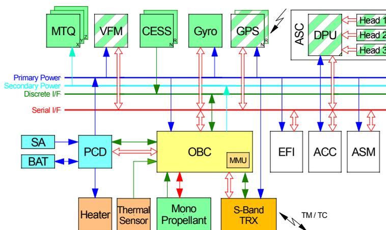
*Figure 3.3: swarm Overall Electrical Architecture*
