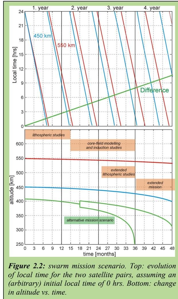
**Figure 2.2:** swarm mission scenario. Top: evolution of local time for the two satellite pairs, assuming an (arbitrary) initial local time of 0 hrs. Bottom: change in altitude vs. time.
