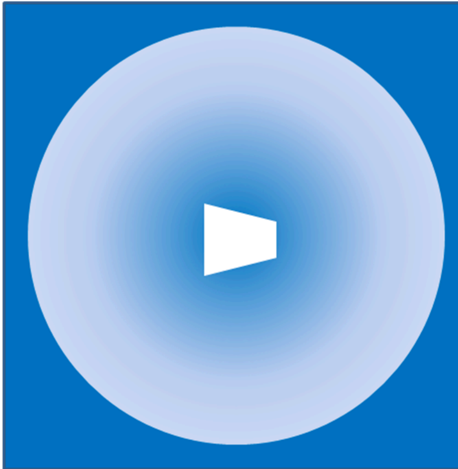
Figure 3: Schematic aperture stop, located directly upstream from the aperture plate, is used to limit the beam illuminated in both radius and azimuth in the baseline approach. The aperture
