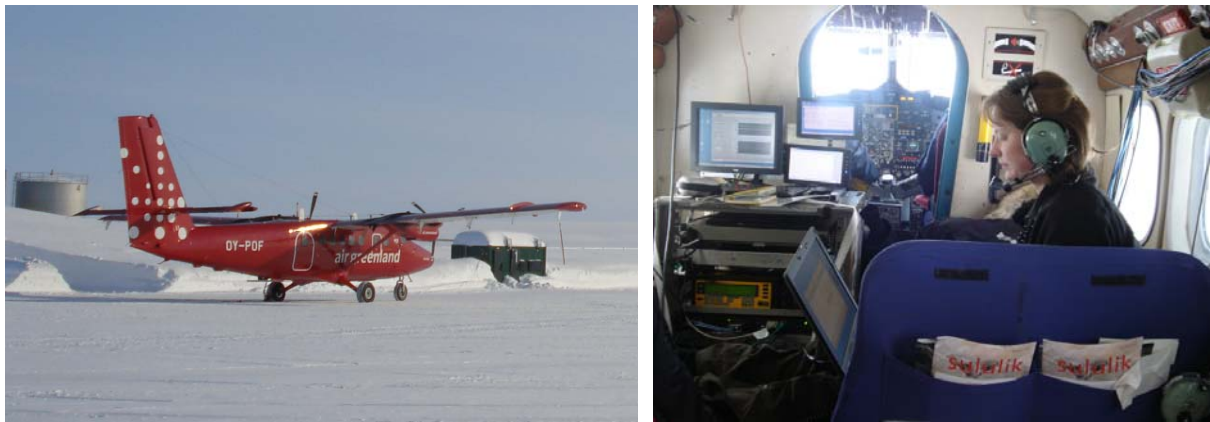
Air Greenland Twin-Otter at Station Nord, April 2008. ASIRAS radar antenna seen just behind door.
