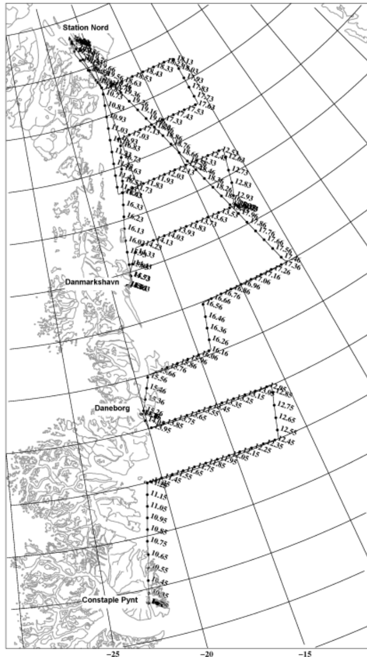
Fig. 14. Actual flight lines on the NE Coast. No lidar measurements were possible on the southern lines due to fog, but measurements were done instead with the 13 GHz ASIRAS interferometric radar, yet to be finally processed.
