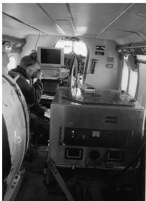
Fig. 4. Internal view of aircraft installation looking forward in cabin. Ferry tank to the left, LCR gravimeter to the right, and electronics rack in background.
