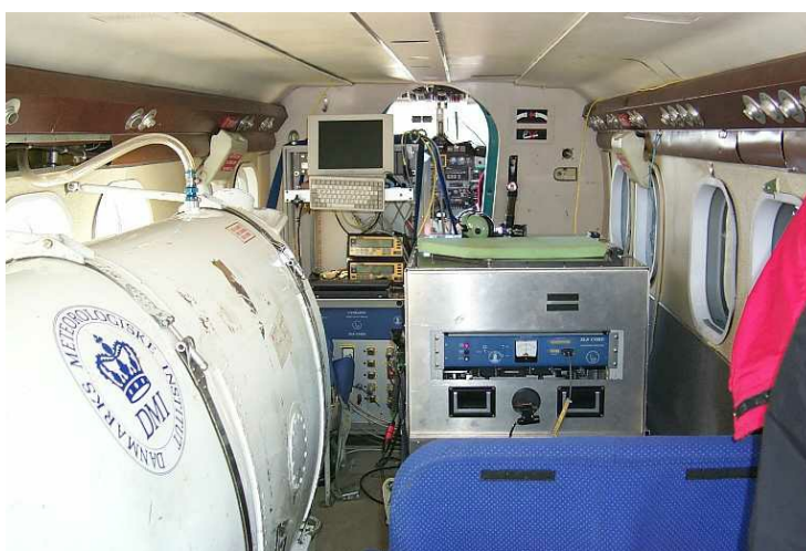
Cabin interior view (1999). Ferry tank on left, gravimeter on right, rack in background
