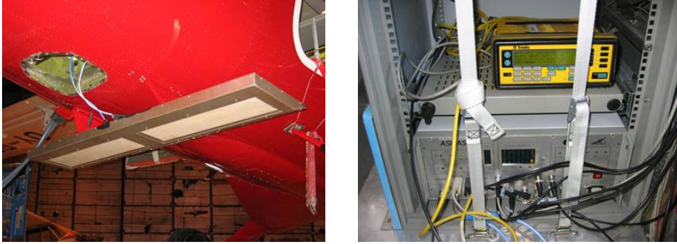
Photos of the ASIRAS installation.
